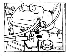
remove sealing cap (shaded) from charcoal canister
