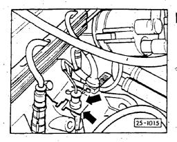
If the CO value is less than 0.3 or more than 3.0% volume when the oxygen sensor is disconnected, adjust the CO as follows:
