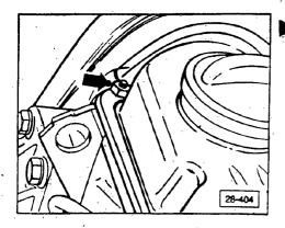
marking on camshaft sprocket must align with cylinder head cover (arrow)
