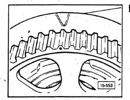
dot on camshaft must line up with marking on cylinder head cover
