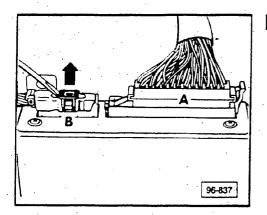
pry open secondary lock (black) of control unit harness connector B and remove
