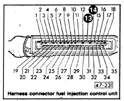
If the fault lamp does NOT light up with "ignition ON," but only after bridging the top of the fuel pump relay terminals, check wiring between terminal 3 of electronic ignition control unit and terminal 13 of fuel injection control unit according to wiring diagram.
