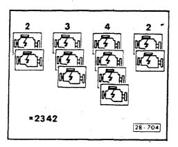
Fault warning lamp 🖅 in instrument cluster will blink a code consisting of groups of one, two, three or four flashes
